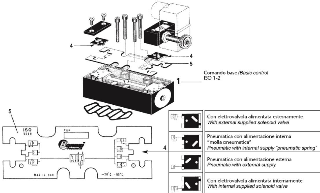
**DIAGRAM FOR ASSEMBLING OF MANIFOLDS**
