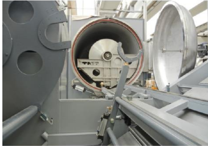
Detail of autoclave with its door of automatic opening (realized in diameters also higher than two meters, for volumes that can reach up to 13thousands litres).
