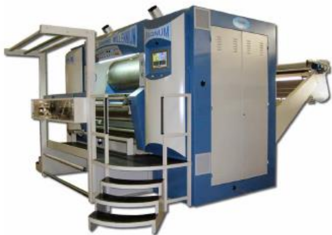
The series PF 3000 includes n° 4 models with autodave from 1.200 to 2.200 mm of diameter.
