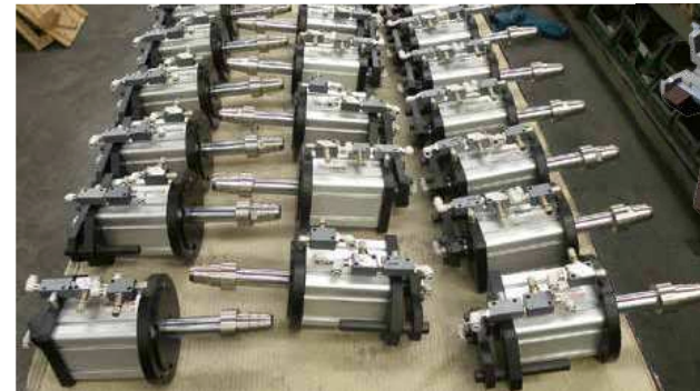
Double acting compact cylinder realized by Bonesi Pneumatik for Comes.
