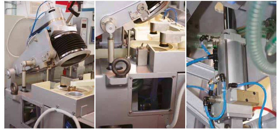
A pneumo-hydraulic control unit on a machine for production of ophthalmic lens.
